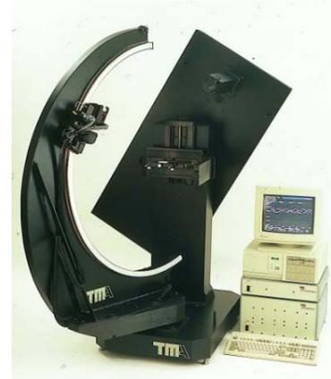
The **TASC Scatterometer** above right is essentially a CASI that takes hemispherical measurements with manually changed apertures. UV, visible, mid-IR and broadband systems have been built. A single red laser system is \$250,000.
