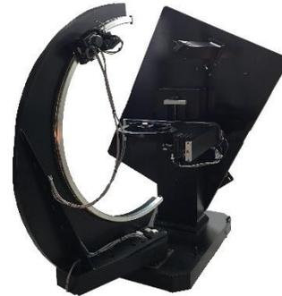
The **TASC** Scatterometer above right is essentially a CASI that takes hemispherical measurements. UV, visible, mid-IR and broadband systems have been built. A single red laser system is about \$283,000.
